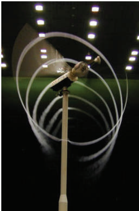
Wind Turbine Tip Speed Visualization using smoke at the National Renewable Energy Laboratory (NREL).
